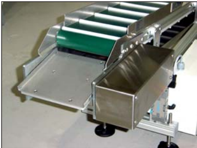
Spreading Discharge Chute
