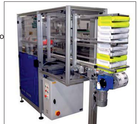
Stacking plastic trays at 20 trays per minute
