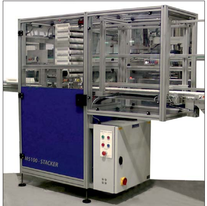
Stacking plastic trays at 20 trays per minute
